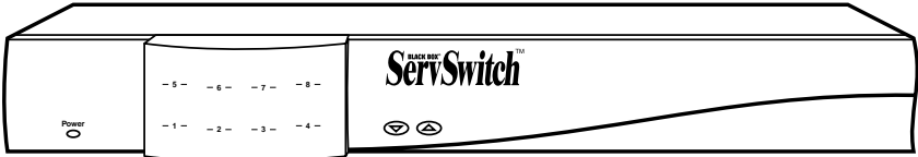
Figure 2-2. The front panel of a slimline 8 to 1 ServSwitch (KV3108SA-R4).
